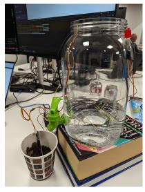
This butt uses sensors to read the water level, water temperature and soil moisture level which is tied together with a UI dashboard.
