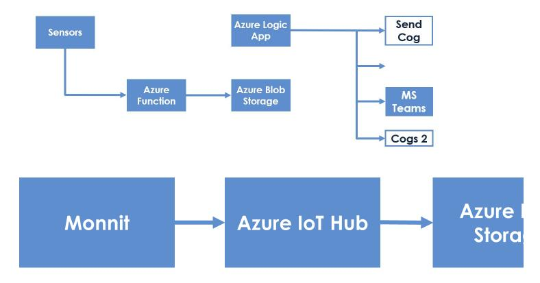
This system works by picking up data from the sensors, filtering it through an Azure IoT hub, blob storage and an Azure function to clean the data, make it understandable then posts to MS Teams as recognition. This then can also filter into other programmes such as rewards (cogs) and recognition (shout out).
